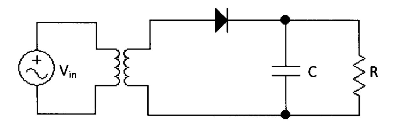
Sketch the out put waveforms across resistor R, with and without capacitor C.
