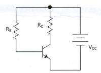
where  $V_{CE} = 8V$ ,  $R_C = 3k\Omega$ , and  $V_{CC} = 15V$ .
