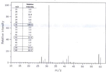
The above data obtained from electron ionization mass spectrometry for the molecule of 1-propanolol.
